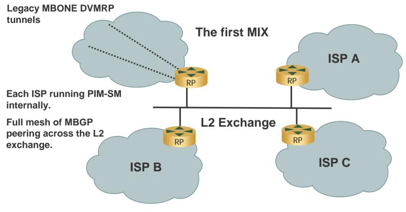
BUT, RPs MUST be on the exchange, and PIM-DM run on the MIX interfaces to flood S,G info to all other RPs
